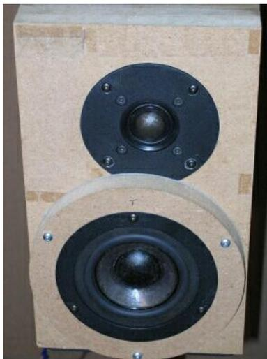
Photo 5: Untreated baffle
