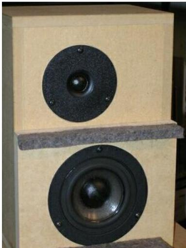
The piece of felt shown in *Photo 2* is the simplest one and is always useful. It does not necessarily need to be the full width of the baffle to be effective. The aesthetics also are not bad. All systems, including flat baffles, would benefit from this.
