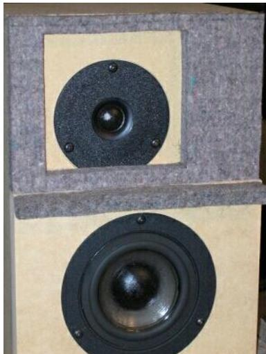
Photo 3: Adding felt block to tweeter face
