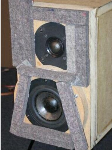
Photo 6 shows the full treatment of felt that was the most effective. It's not pretty, but it works well. I will be replacing the ring and felt, however, with a rectangular piece as shown on the first box.
